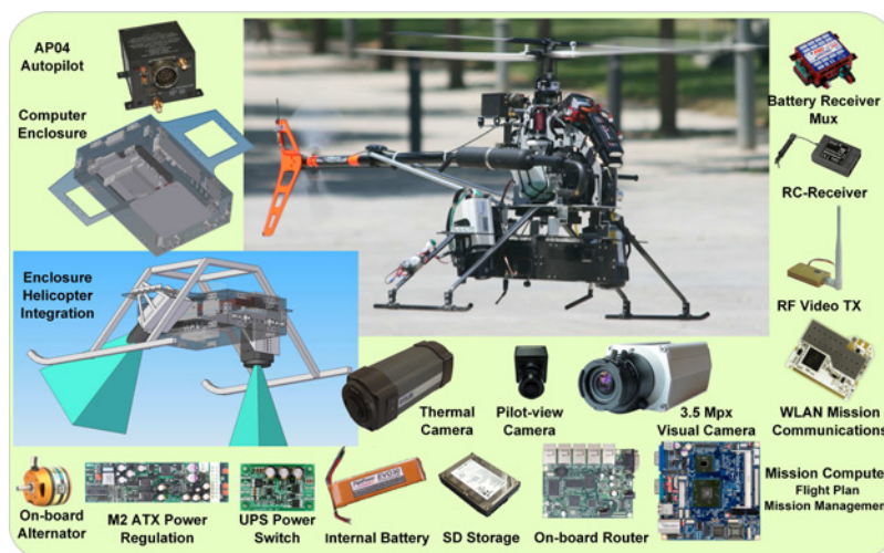
Fig. 15 Sky-Eye UAS prototype based on the AP04 autopilot and the combination of VAS and USAL architecture.
